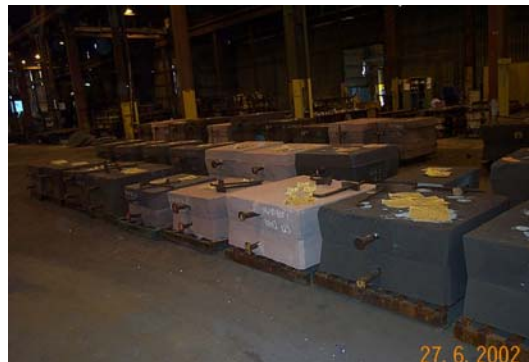
Casting moulds – dark from reclaimed sand, light from new sand
